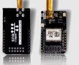
"tGPS BoB " is a formative with a microBUS structure. It is an effective and easy solution for adding GPS functionality to your design.It features the Telit SL869 - V2S module, a SMA connector for an GPS antenna also it has two LEDs for PPS and PWR. tGPS BoB can be interfaced with the target board microcontroller via microBUS UART ( Rx, Tx), lines. It has a LED diode in order to power indicator.it can function on 3.3 V power supply only.
